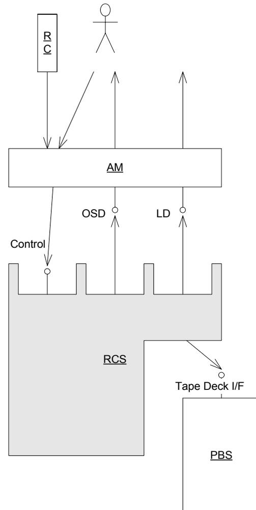
Figure 4. RCS adapted for DVD+RW has removed input code, OSD, LD. AM provides now that functionality exporting the same interfaces. The input interface may change if the proposed mechanism needs more control of AM over RCS or vice versa. Also the tape deck part is removed and replaced by PBS functionality. In our exercise, we will not take this last fact into consideration.
