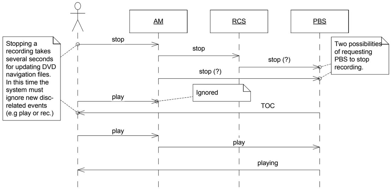
Since RCS can control PBS as tape deck, it can send stop request directly to PBS (depending on the mechanism chosen).
