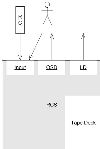
Figure 3. Original RCS communicates directly with the user through its own RC Controller, Local Keyboard, On-Screen Display, and Local Display.
